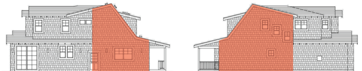
Unbroken two-story wall is not consistent with Residential Design Guideline 3.3.3
